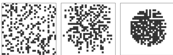
Fig. 7 Example of Monte Carlo calculation of equilibrium state of a plasma. At low temperature, after 10^5 steps, the initial uniform distribution of low-(black) and highly-(white) charged ions becomes circular to minimize the surface area.
