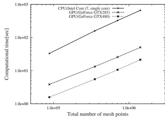
Fig. 4 Computational time using a CPU (Core i7) and two GPUs (GTX285 and GTX480). The horizontal axis is the total number of mesh points ( $NX \times NY \times NZ$ ).
