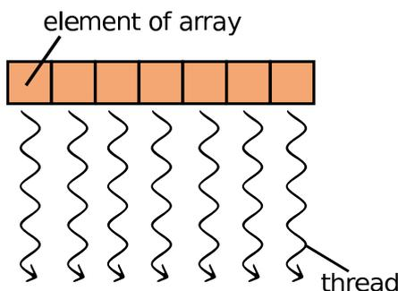
Fig. 1 Mapping of each array element to the corresponding thread on the GPU.
