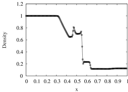
Fig. 3 Density profile at  $t = 0.1$ . The solid line is the solution of the CPU code. The squares are the solution of the GPU code.
