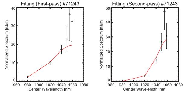
Fig. 4 Result of fitting of first- and second-pass signals to the Thomson spectrum. + denotes the measured value and the red line denotes the fitting result. The error bars are plotted. Each wavelength signal is normalized by its wavelength-integrated responsivity.
