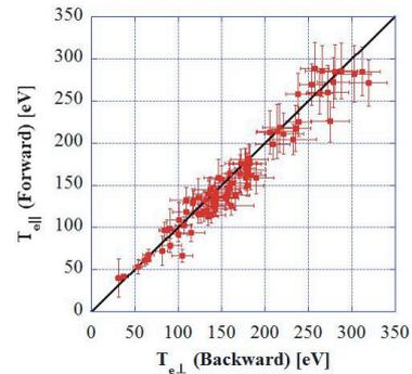
Fig. 5 Relationship between  $T_{e\perp}$  and  $T_{e\parallel}$  for high-density plasmas.
