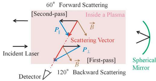
Fig. 2 Schematic diagram of temperature anisotropy measurement by double-pass Thomson scattering scheme on TST-2.
