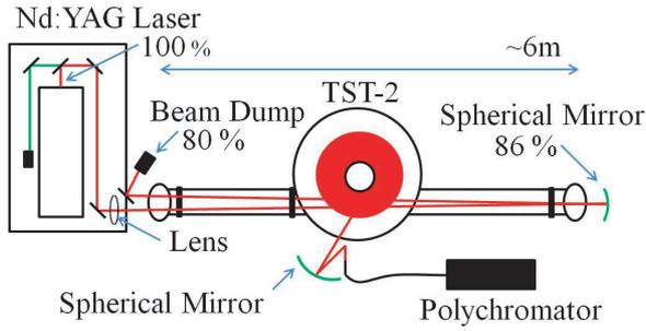
Fig. 1 Schematic diagram of the double-pass Thomson scattering system on TST-2.
