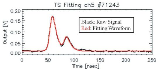
Fig. 3 Typical waveform of double-pass Thomson scattering measurement. The black line denotes the raw signal and the red line denotes waveform fitting.
