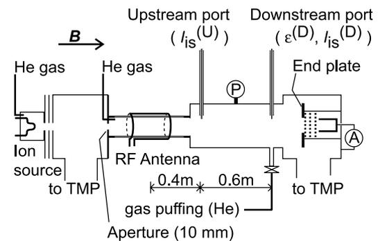
Fig. 1 Schematic representation of the DT-ALPHA device.
