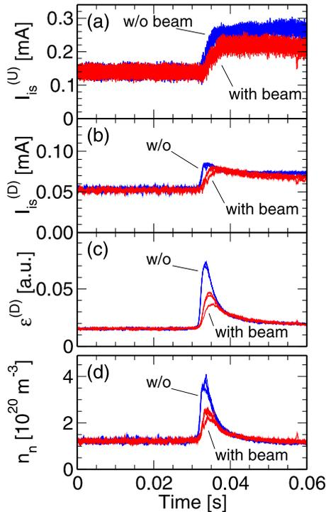
Fig. 2 Time responses of a helium plasma to helium gas puffing without and with helium beam injection. Vertical axes represent (a) ion saturation current at the upstream port  $I_{is}^{(U)}$ , (b) ion saturation current at the downstream port  $I_{is}^{(D)}$ , (c) line emission intensity at the downstream port  $\varepsilon^{(D)}$ , and (d) deduced neutral density  $n_n \sim \varepsilon^{(D)}/I_{is}^{(D)}$ . Three traces for each condition illustrate the reproducibility between discharges.
