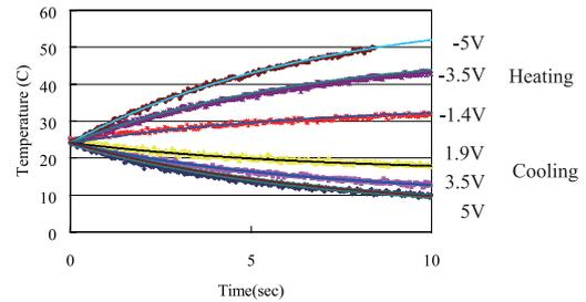
Fig. 4 Assumed time constant of the Peltier element (the initial temperature is ambient).
