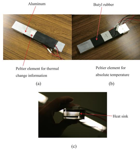
Fig. 2 Proposed thermal display (a) Peltier element for thermal change information, (b) Peltier element for absolute temperature, (c) inside the device.
