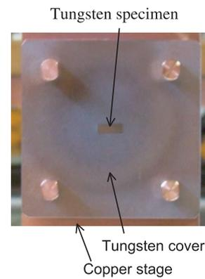
Fig. 6 One of four specimens mounted on a copper stage set around 1530 mm from the electrode. PM tungsten specimen of  $10 \times 5 \times 1$  mm<sup>3</sup> is fixed between the copper stage and tungsten cover. Irradiation area on specimen is limited to  $8 \times 3$  mm<sup>2</sup>. Surface color of the tungsten cover became gray after irradiation.
