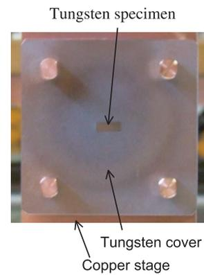
Fig. 6 One of four specimens mounted on a copper stage set around 1530 mm from the electrode. PM tungsten specimen of  $10 \times 5 \times 1 \text{ mm}^3$  is fixed between the copper stage and tungsten cover. Irradiation area on specimen is limited to  $8 \times 3 \text{ mm}^2$ . Surface color of the tungsten cover became gray after irradiation.
