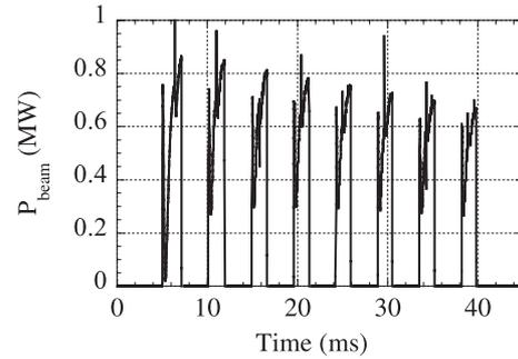
Fig. 2 Time evolution of repetitive short-pulse ion beam obtained spontaneously in the case of brakedown.
