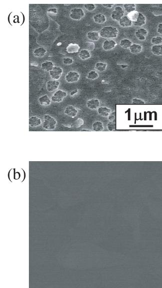
Fig. 7 Tungsten surface images obtained by SEM after beam irradiation: (a) long pulse irradiation [11] and (b) repetitive short-pulse beam irradiation (it is difficult to identify the change due to the limitation of contrast).
