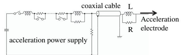
Fig. 3 Acceleration power supply system after modification. Inductance  $L$  is inserted between the electrode and long coaxial cable from the power supply.
