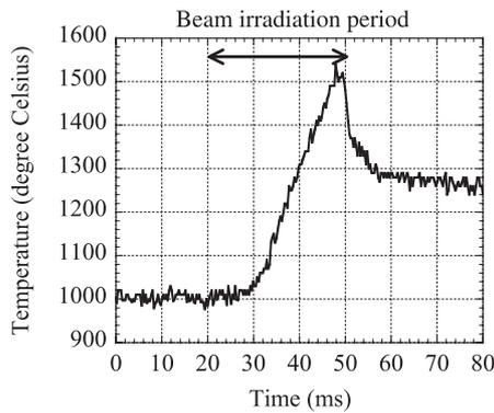
Fig. 8 Time evolution of tungsten surface temperature measured with fast optical pyrometer with a sensitivity of more than 1,000 degree Celsius.
