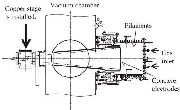
Fig. 1 Ion beam system.
