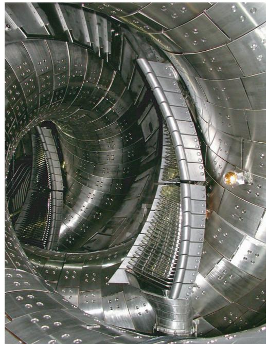
Fig. 1 Two sets of ICRF antennas are set on the outer side of toroid in the LHD vacuum chamber. They are positioned in front of the superconducting helical windings.
