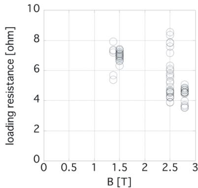
Fig. 7 Loading resistance versus strength of magnetic field. Data are from the 3.5U antenna at 38.47 MHz without NBI. Line-averaged electron density is kept between  $0.5$  and  $1.5 \times 10^{19} \text{ m}^{-3}$ . Antenna gap is kept between 8 and 11 cm.
