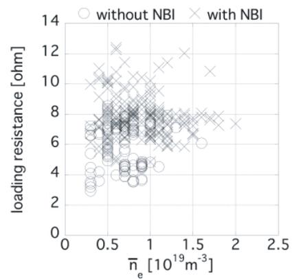
Fig. 5 Loading resistance versus line-averaged electron density. Data are from the 3.5U antenna at 38.47 MHz. Antenna gap is kept between 8 and 11 cm.
