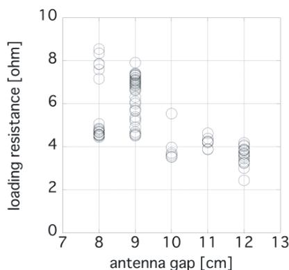
Fig. 4 Loading resistance as a function of the gap between the antenna surface and the LCFS. Data are from the 3.5U antenna, at 38.47 MHz, without NBI. Line-averaged electron density is kept between  $0.5$  and  $1.5 \times 10^{19} \text{ m}^{-3}$ .
