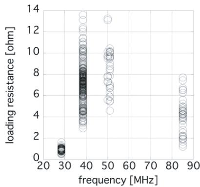
Fig. 3 Loading resistance versus wave frequency. Data are from the 3.5U antenna. Antenna gap is kept between 8 and 11 cm.
