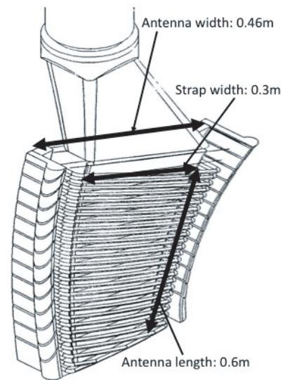
Fig. 2 Schematic drawing of the radiating part of the antenna.
