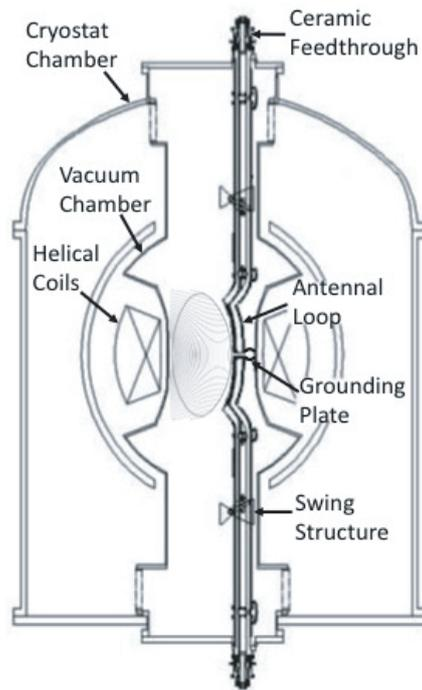
Fig. 1 Cross-sectional view of LHD and ICRF antennas. Center of the torus is located on the left. Flux surfaces and mod-B contours are also plotted.
