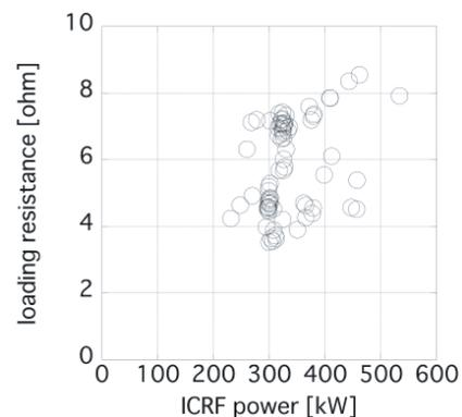
Fig. 6 Loading resistance versus injected ICRF power. Data are from the 3.5U antenna at 38.47 MHz without NBI. Line-averaged electron density is kept between  $0.5$  and  $1.5 \times 10^{19} \text{ m}^{-3}$ . Antenna gap is kept between 8 and 11 cm.
