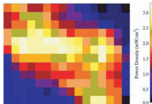
Fig. 6 Sample radiated power density image from IRVB at LHD Port 10-O (shot 97279).
