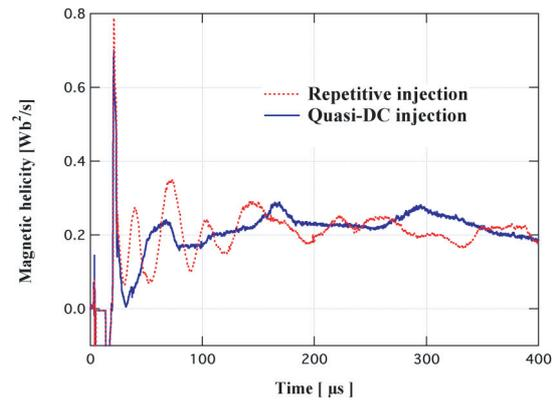
Fig. 8 Time derivative of helicity injected from MCPG.
