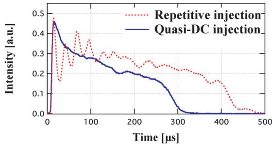
Fig. 6 Time evolution of helium ion (HeII) spectrum intensity.
