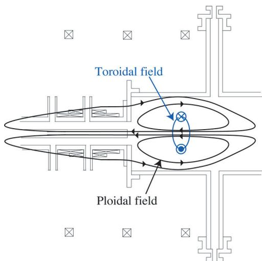
Fig. 4 Ejected spheromak from MCPG.
