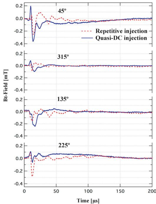
Fig. 9 Time history of toroidal field measured in the poloidal cross section at  $z = 165$  mm.
