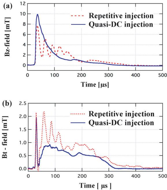
Fig. 7 Time development of (a) poloidal (vertical) and (b) toroidal magnetic field density observed by the internal probe array.
