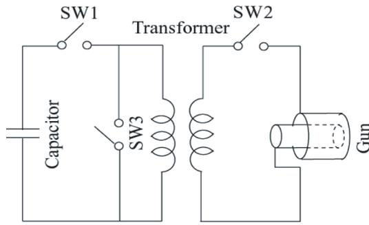
Fig. 2 Transformer-coupled discharge circuits.
