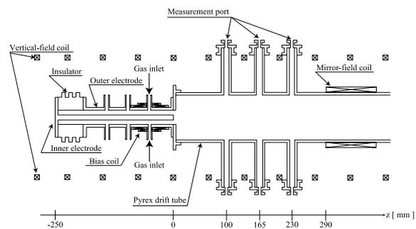
Fig. 1 Typical schematic diagram of experimental set up.
