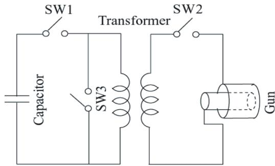
Fig. 2 Transformer-coupled discharge circuits.
