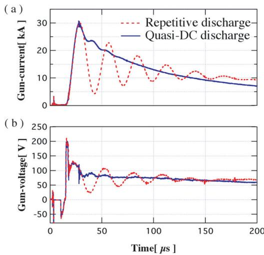
Fig. 3 Typical waveform of (a) gun current and (b) gun discharge voltage on the MCPG.
