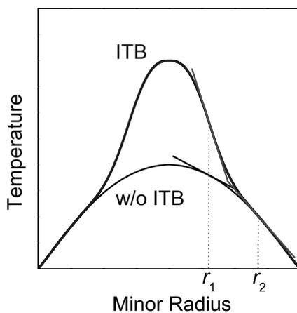
Fig. 2 Schematic of typical temperature profiles of ITB plasma and L-mode plasma. Temperature gradients in the ITB region ( $r_1$ ) and peripheral region ( $r_2$ ) are also shown.
