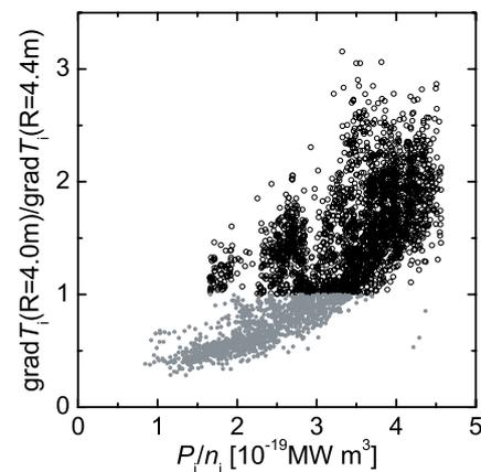
Fig. 3 Ratio of ion temperature gradient in the core ( $R = 4.0$  m; normalized minor radius  $r/a \sim 0.42$ ) and that at the periphery ( $R = 4.4$  m;  $r/a \sim 0.88$ ) as a function of total ion heating power normalized by the average ion density. Plasmas with and without an ion ITB are indicated by open (black) and closed (gray) circles, respectively.
