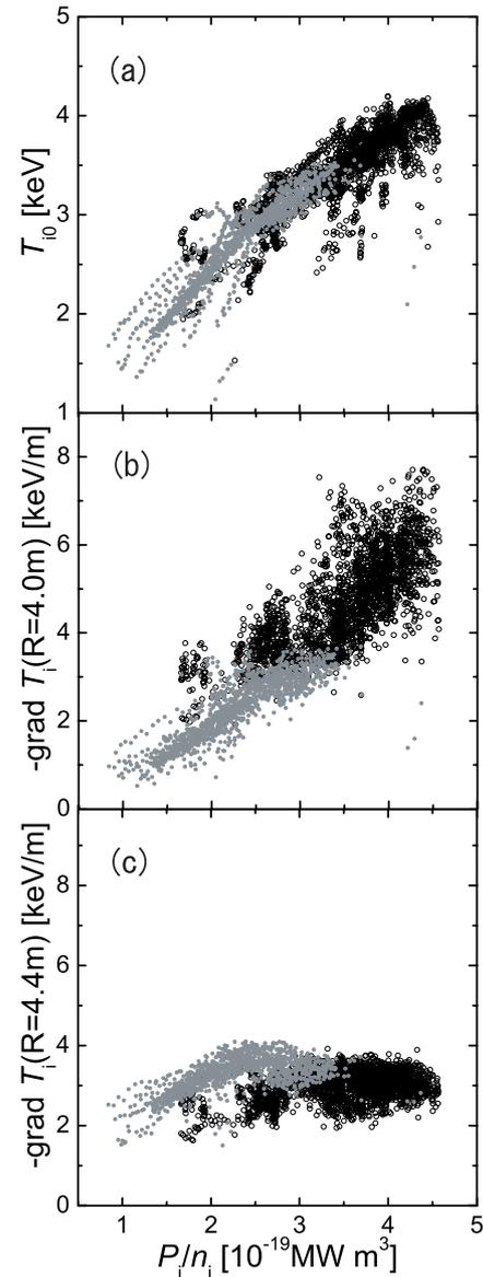
Fig. 5 (a) Central ion temperature, (b) gradient of ion temperature at  $R = 4.0 \text{ m}$  ( $r/a \sim 0.42$ ), and (c) that at  $R = 4.4 \text{ m}$  ( $r/a \sim 0.88$ ) as a function of ion heating power normalized by average ion density.
