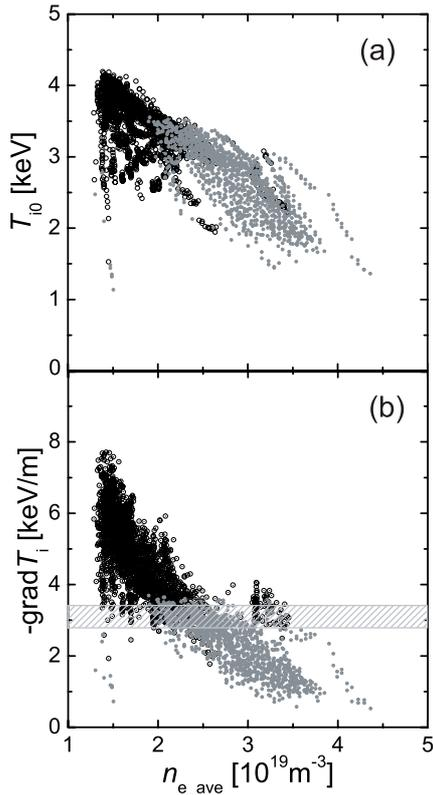
Fig. 4 (a) Central ion temperature and (b) temperature gradient at  $R = 4.0 \text{ m}$  ( $r/a \sim 0.42$ ) as a function of line-averaged electron density. Plasmas with and without an ion ITB are indicated by open (black) and closed (gray) circles, respectively.
