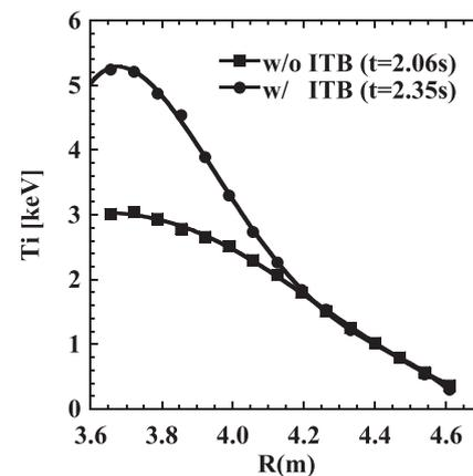
Fig. 1 Ion temperature profile of NBI-heated plasma with ITB (circles) and without ITB (squares).
