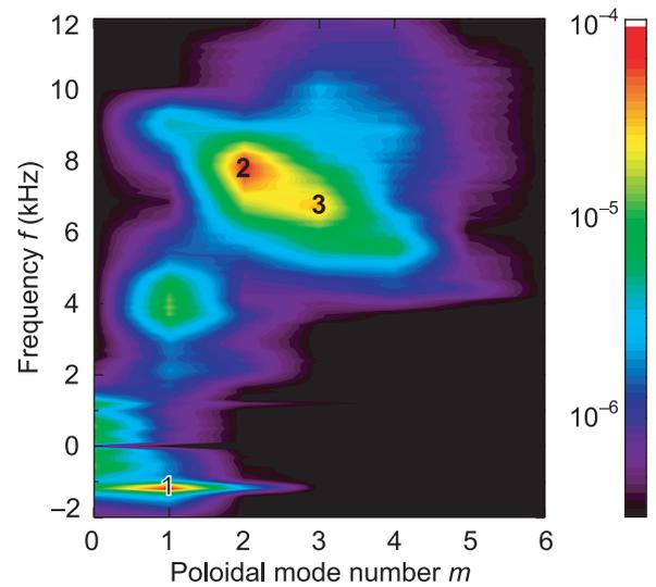
Fig. 3 2D power spectrum of the ion saturation-current fluctuation observed in Fig. 2(a). Frequencies and poloidal mode numbers of three pronounced modes labeled “1”, “2”, and “3” are  $(f, m) = (-1.2 \text{ kHz}, 1)$ ,  $(7.8 \text{ kHz}, 2)$ , and  $(6.6 \text{ kHz}, 3)$ . These three modes satisfy the matching conditions.
