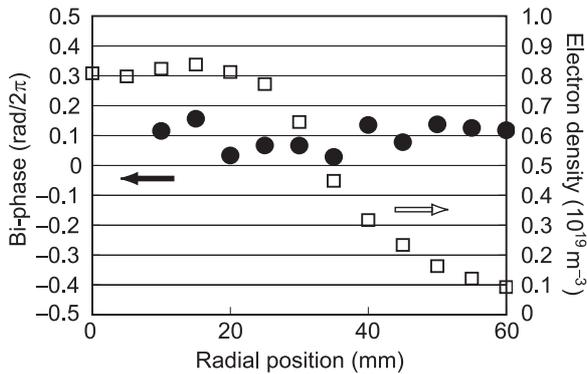
Fig. 4 Radial profile of the biphase between modes 1, 2, and 3 (closed circles).  $Z_1 = Z(f_1, m_1)$ , measured with 64-channel poloidal probe array (reference signal), and  $Z_2 = Z(f_2)$  and  $Z_3 = Z(f_3)$ , measured with a radially movable probe, were used for the calculation. Result indicates that the poloidally localized structure is almost radially independent. Open squares indicate the electron density profile.
