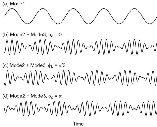
Fig. 1 Drawing showing ideal cases of the phase relationship between three coupling modes, 1, 2, and 3. (a) Mode 1 ( $-1.2$  kHz) and (b–d) the envelope generated by modes 2 ( $7.8$  kHz) and 3 ( $6.6$  kHz). Biphases of the three coupling modes are (b)  $0$ , (c)  $\pi/2$ , and (d)  $\pi$ .
