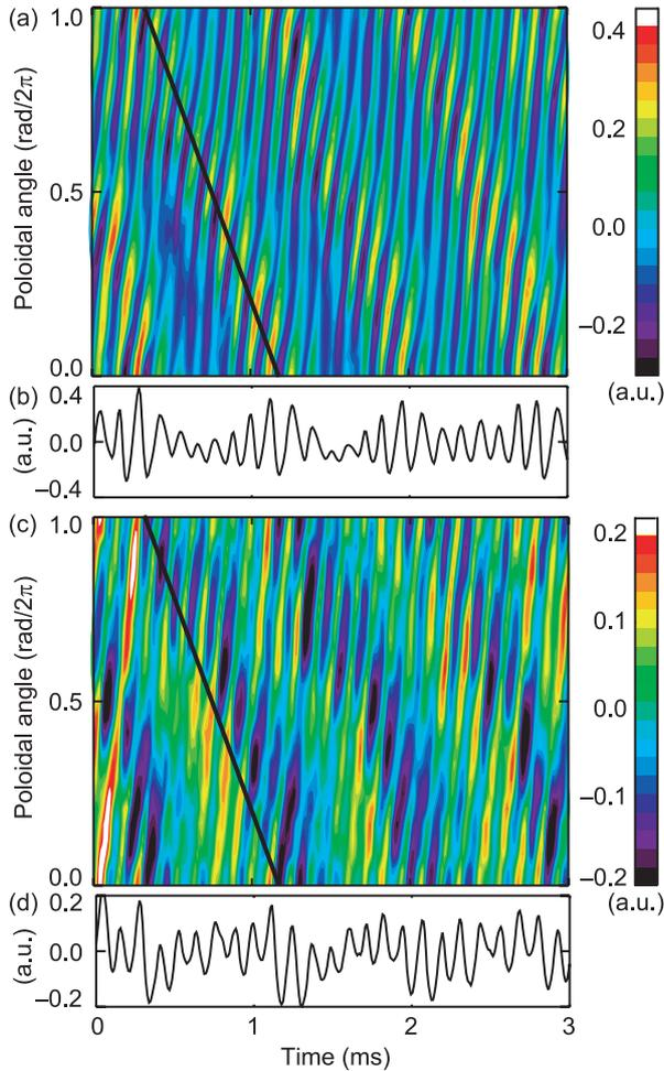
Fig. 2 Spatiotemporal waveforms of ion saturation-current fluctuations measured at radii of (a) 40 mm with a 64-channel poloidal probe array and (c) 20 mm with a 24-channel poloidal probe array. (b), (d) Temporal waveforms of (a), (c) at zero poloidal angle positions. Black lines in (a) and (c) indicate the same timings and positions. Both lines trace the high-amplitude regions of the poloidally localized structures.
