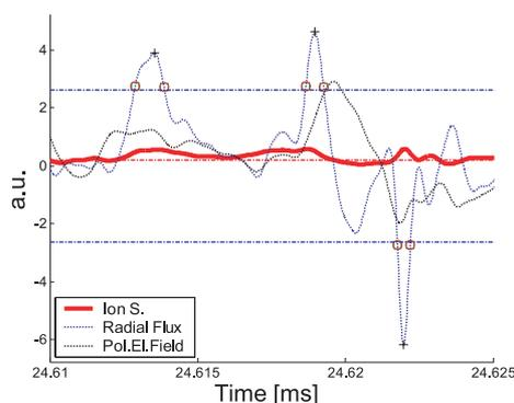
Fig. 2 Time series of sampled signals with mean ion saturation current and 2.5RMS thresholds of radial flux in horizontal lines.
