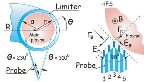
Fig. 1 Schematics showing the movable 5-electrode Langmuir probe measurements on the poloidal cross-section of FT-2.
