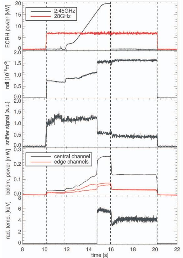
Fig. 2 From above: Time traces of the forward power of the 2.45 GHz and the 28 GHz microwave system, the line-integrated density, the signal of the non-absorbed 28 GHz stray radiation, a central (black) and two edge channels (red) of the bolometer camera and a central channel of EBE diagnostic measuring the radiation temperature for the helium discharge #30344.
