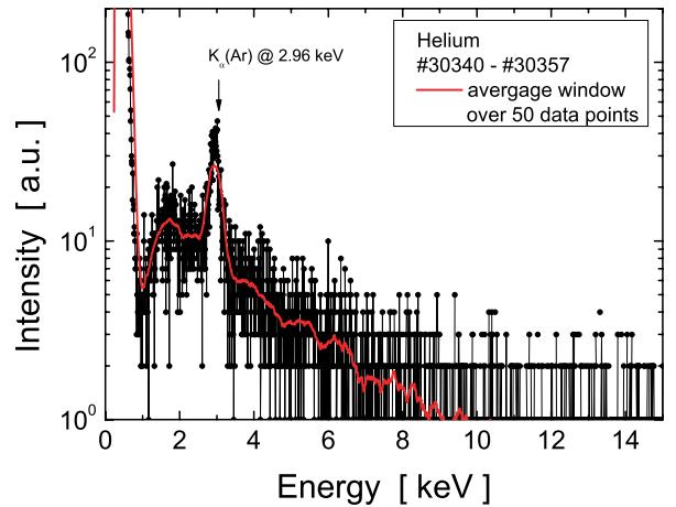
Fig. 4 Soft X-ray signals during the OXB heated plasma phase averaged over 15 identical discharges and for comparison a 10 keV curve representing the supra-thermal electrons.
