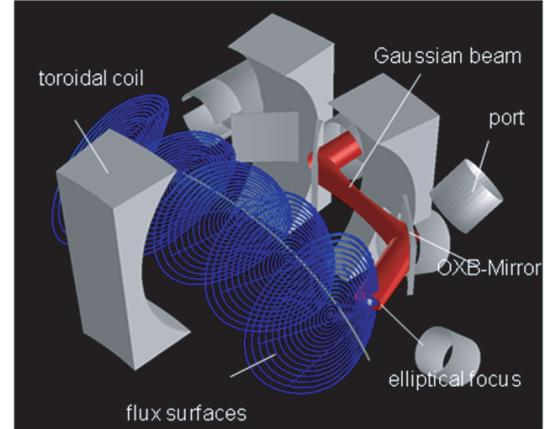
Fig. 1 Setup of the focussing mirror system inside the plasma vessel. The beam trajectory is indicated in red, the magnetic flux surfaces in blue.
