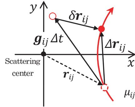
Fig. 3 Relative motion for particle pair  $(i, j)$ . Scattering center is at the origin. The change in position of the particle with a mass  $\mu_{ij}$  is  $\Delta \mathbf{r}_{ij}$ . If no interaction occurs, the change in position is  $\mathbf{g}_{ij} \Delta t$  during a time interval of  $\Delta t$ .
