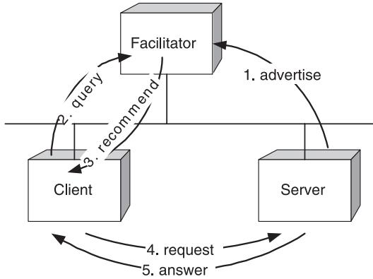
Fig. 3 Recommend-type facilitator model: The facilitator never mediates requests but only recommends the appropriate server to which to send them [13]. It is suitable for a distributed data storage and retrieval system that must transfer many binary large objects (BLOBs) without bottlenecks.
