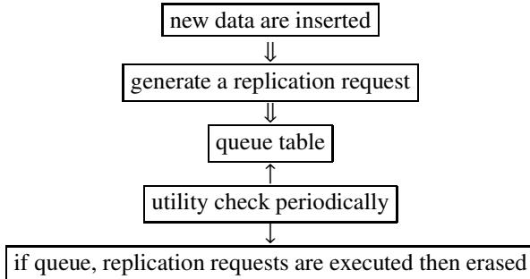
Fig. 5 Replication queuing algorithm between the database table and the utility.
