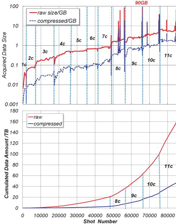
Fig. 1 Data growth in LHD, per-shot size (top) and cumulative amount (bottom): 1c-11c represent annual experimental LHD campaigns. 90 GB/shot is the world record for raw data acquired in one experimental plasma discharge. All acquired data are kept online to be accessible to every collaborator.
