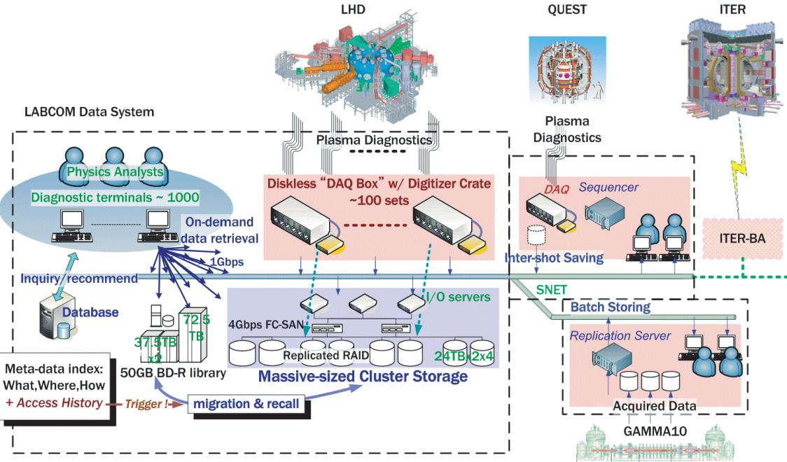
Fig. 4 LABC/X multi-site data system based on SNET: The database at the left end performs the *facilitator* function, and user diagnostic terminals are the data clients. DAQ and I/O servers at both the LHD and SNET sites correspond to the distributed servers in the *facilitator* model.
