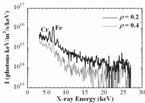
Fig. 2 Abel inverted x-ray energy spectra obtained with soft x-ray PHA assembly installed at the bottom port. Thick and thin lines represent x-ray spectra at  $\rho = 0.2$  and  $0.4$ , respectively.  $K_{\alpha}$  lines from metallic impurities of Cr and Fe are also observed at 5.6 and 6.7 keV, respectively.
