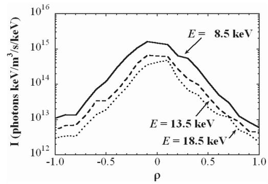
Fig. 3 Radial profiles of Abel inverted x-ray spectra at energies of 8.5, 13.5 and 18.5 keV.
