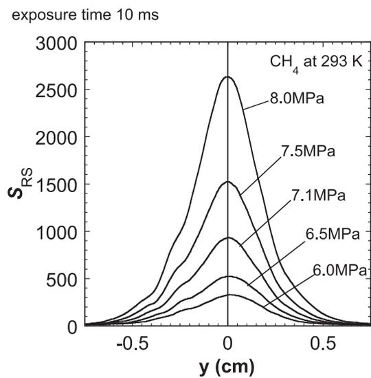
Fig. 5 Typical scatter signal profiles in the case of CH<sub>4</sub>. The direction y is parallel to the laser light. The backing pressure  $P_0$  is scanned from 6.0 MPa to 8.0 MPa, while the gas puff pulse length of 40 ms, the CCD camera trigger timing of 35 ms, and the exposure time of 10 ms are fixed.
