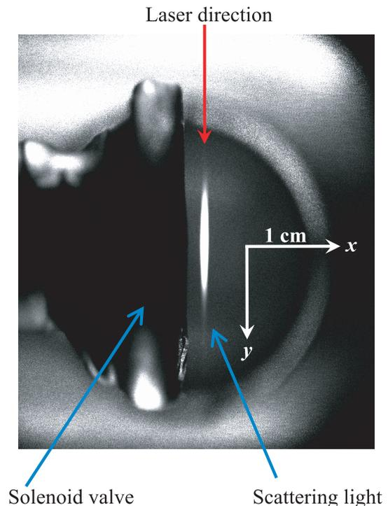
Fig. 3 The scattering light image detected by the CCD camera in the case of  $\text{CH}_4$ . The backing pressure is 8.0 MPa, and the exposure time is 10 ms. The laser beam direction ( $y$ ) is perpendicular to the gas flow ( $x$ ).
