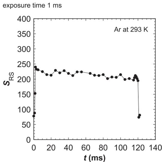
Fig. 4 Typical temporal behavior of the scattering signal intensity. The working gas is Ar and the backing pressure is 7.1 MPa.
