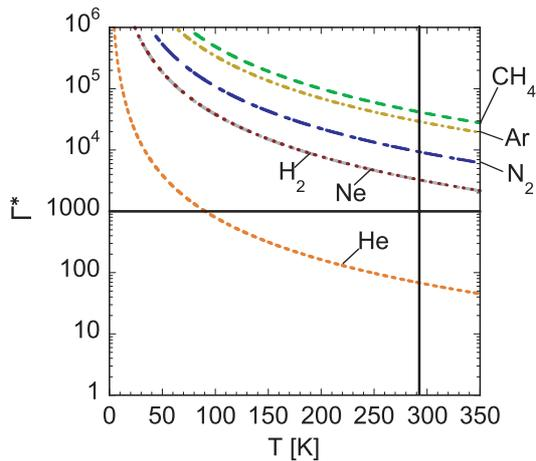
Fig. 1 Calculated results of the scaling parameter  $\Gamma^*$ , where  $d = 500 \mu\text{m}$ ,  $\alpha = 45^\circ$ ,  $P_0 = 4 \text{ MPa}$ . The gasses except helium satisfy the condition for massive condensation of  $\Gamma^* > 1000$  at room temperature (293 K).
