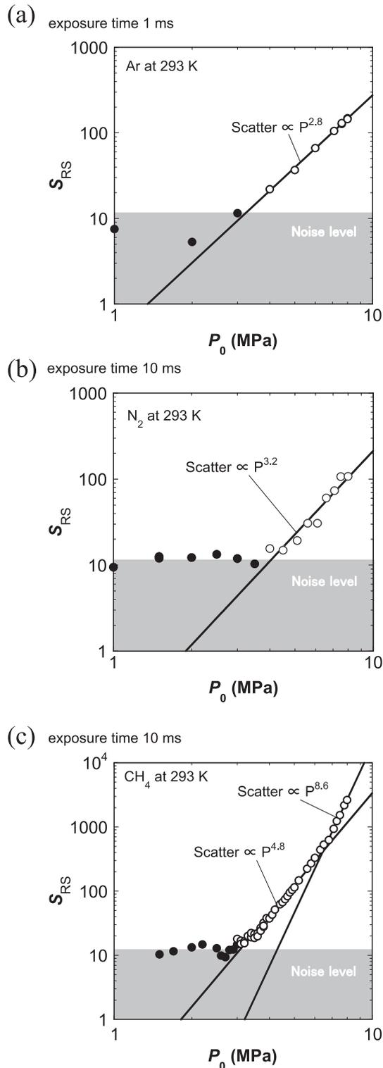
Fig. 8 Peak scattered signal as a function of the backing pressure in the cases of (a) Ar, (b)  $N_2$  and (c)  $CH_4$ . Closed circles denote the signals under the noise level. Regression analysis has been done using the data points denoted by open circles.
