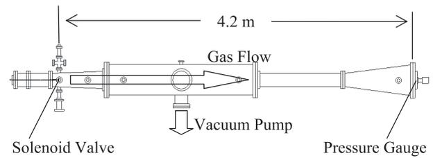
Fig. 2 Schematic of the experimental setup. The distance from the solenoid valve to the baratron pressure gauge is 4.2 m. Inside the chamber is pumped to less than  $10^{-4} \text{ Pa}$ . The laser is set inside the chamber.
