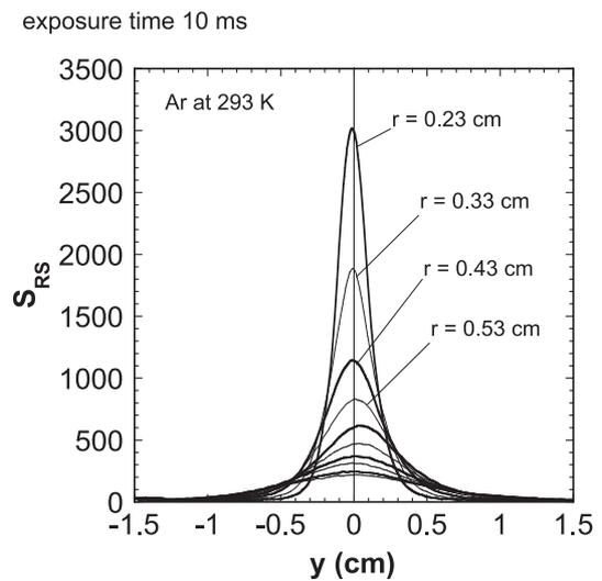
Fig. 6 Scatter signal profiles in the case of Ar, where the distance from valves to laser light is varied from 0.23 cm to 1.0 cm. The direction y is parallel to the laser beam.
