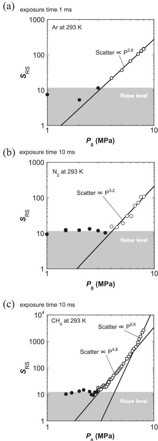
Fig. 8 Peak scattered signal as a function of the backing pressure in the cases of (a) Ar, (b)  $N_2$  and (c)  $CH_4$ . Closed circles denote the signals under the noise level. Regression analysis has been done using the data points denoted by open circles.
