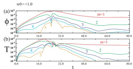
Fig. 5 Time evolution of Fourier components of  $\Phi$  and  $T$  for various azimuthal mode numbers  $m$  at  $x = 1/2$ .
