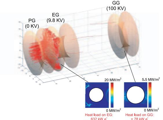
Fig. 4 EAMCC simulation of the beam in the 100 kV accelerator: the particle trajectories and stripping reaction are simulated with a Monte Carlo approach in a domain with electrical and magnetic fields. The power corresponding to the whole accelerator (1280 beamlets) is reported.
