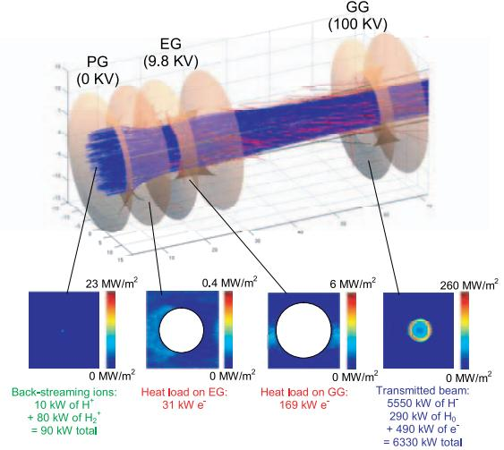
(b) Simulation of co-extracted electrons
