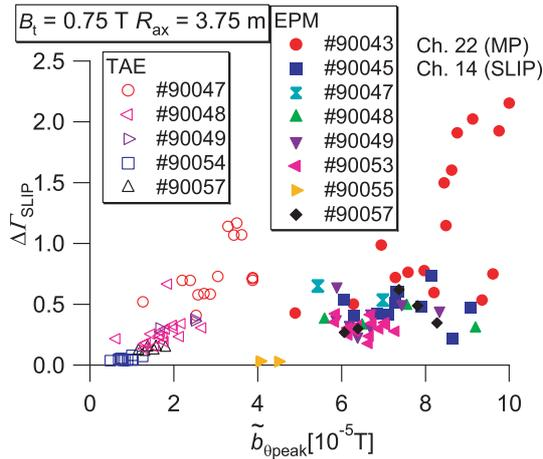
Fig. 3 Increment of SLIP signal as a function of the amplitude of TAE/EPM fluctuations at the probe position. Data points obtained in multi-shots of #90043, #90045, #90047, #90048, #90049, #90053, #90054, #90055, and #90057 are plotted.
