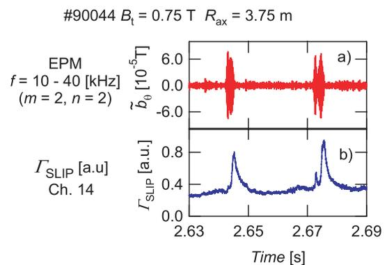
Fig. 2 Typical time traces of EPM fluctuation and SLIP signal in the configuration of  $R_{ax} = 3.75$  m at  $B_t = 0.75$  T (CCW). (a)  $m/n = 2/2$  EPM, and (b) SLIP signal measured with a PMT (Larmor radius/pitch angle is about 100 mm / 35 degrees).
