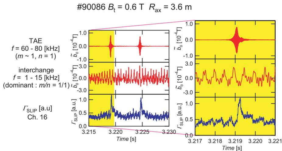
Fig. 1 Typical time traces of magnetic fluctuations of TAE and interchange modes, and SLIP signal in the configuration of  $R_{ax} = 3.6$  m at  $B_t = 0.6$  T (CCW direction). (a)  $m \sim 1$ ,  $n = 1$  TAE fluctuation, (b)  $m/n = 1/1$  interchange modes, and (c) SLIP signal measured with a PMT.
