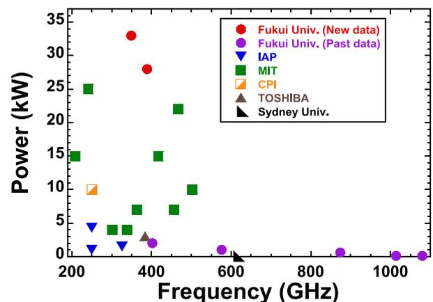
Fig. 2 Radiation power achieved as a function of frequency, for second harmonic gyrotrons.
