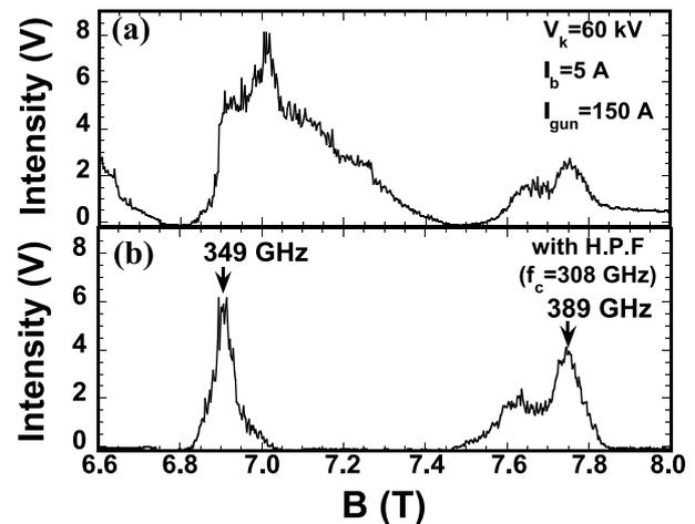
Fig. 1 Dependence of radiation intensity on the magnetic field strength at the cavity: (a) without a high pass filter, and (b) with a high pass filter.
