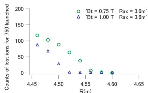
Fig. 3 Counts of energetic ions that are lost from the plasma core region and reach the LIP, where 750 particles are launched from the probe, having various energies and pitch angles. The configuration is  $R_{ax} = 3.6$  m. The results at  $B_t = 0.75$  and 1 T are shown by circles and triangles, respectively.
