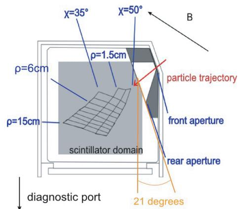
Fig. 6 Schematic view of the probe head and expected arrival area of energetic ions. Expected hit point area of lost ions having the range of 1.5 to 15 cm for gyroradius and 35 to 50 degrees.
