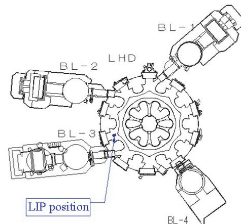
Fig. 1 Top view of LHD where NB injectors and a newly designed LIP are installed. The direction of both BL-1 (180 keV) and BL-3 (180 keV) are in operation to be co- or counter-, depending on the direction of  $B_t$ . On the other hand, BL-2 (180 keV) is in operation to the direction opposite to BL-1 and BL-3. BL-4 is used for perpendicular injection. The position of LIP head is marked near BL-3.
