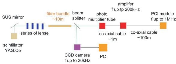
Fig. 7 The block diagram of the signal transfer system and the data acquisition system of the LIP.
