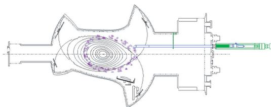
Fig. 5 Schematic view of the LIP placed at the innermost position. The distance between the outermost surface of ergodic layer and the probe head is 120 mm. Triangles designate an example of Poincaré plots of the orbits of lost ion with 150 keV energy and 35.0 degrees pitch angle. It can be moved in the horizontal direction by 750 mm per 1.5 min with a pneumatic motor.
