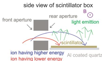
Fig. 4 The side view of the scintillator box. Lost energetic ions pass through two apertures, and then hit the scintillator surface. The strike point provides information about both gyroradius and pitch angle of the lost ion.
