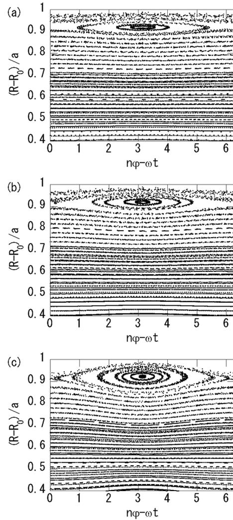
Fig. 5 Poincaré plots for the lower frequency TAE with amplitude (a)  $\delta B_r/B = 10^{-3}$ , and (b)  $\delta B_r/B = 2 \times 10^{-3}$ , and (c)  $\delta B_r/B = 5 \times 10^{-3}$ .
