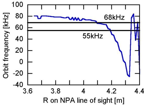
Fig. 4 Blue curve represents energetic-ion orbit frequency with  $m/n = 1/1$  versus major radius of the starting point on the NPA line-of-sight. Black lines denote Alfvén eigenmode frequencies observed in the LHD experiment.
