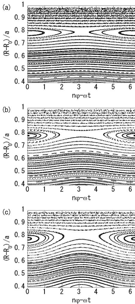
Fig. 6 Poincaré plots for the higher frequency TAE with amplitude (a)  $\delta B_r/B = 5 \times 10^{-4}$ , (b)  $\delta B_r/B = 10^{-3}$ , and (c)  $\delta B_r/B = 2 \times 10^{-3}$ .
