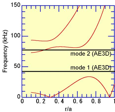
Fig. 2 Alfvén continuous spectra with toroidal mode number  $n = 1$  of the LHD shot #47645. Black lines represent the frequencies of the toroidal Alfvén eigenmodes analyzed with the AE3D code.
