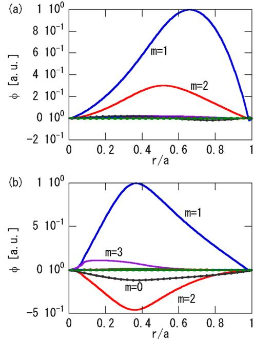
Fig. 3 Spatial profiles of the  $n = 1$  toroidal Alfvén eigenmodes analyzed with the AE3D code for the LHD shot #47645. The frequencies are (a) 42.7 kHz and (b) 79.1 kHz, respectively.
