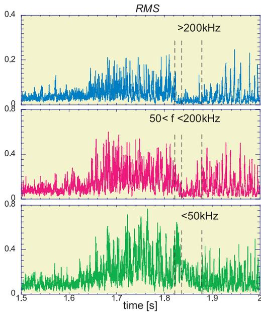
Fig. 3 Time evolution of fluctuation power of reflectometer signal. The frequency component higher than 200-kHz (top), and that higher than 50-kHz and less than 200-kHz (middle), and that less than 50-kHz (bottom), are shown.
