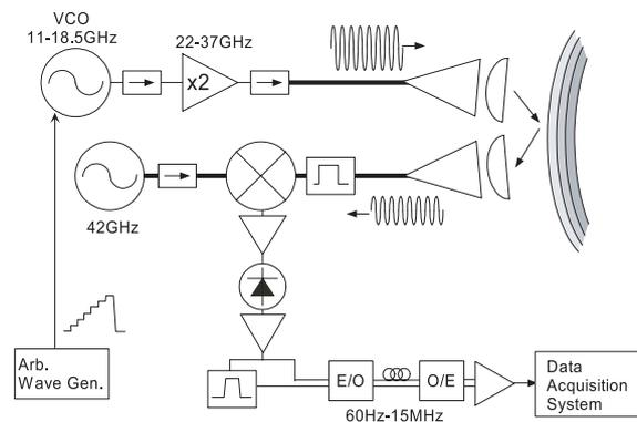
Fig. 4 Schematic view of Frequency Hopping *Ka*-band Reflectometer system.
