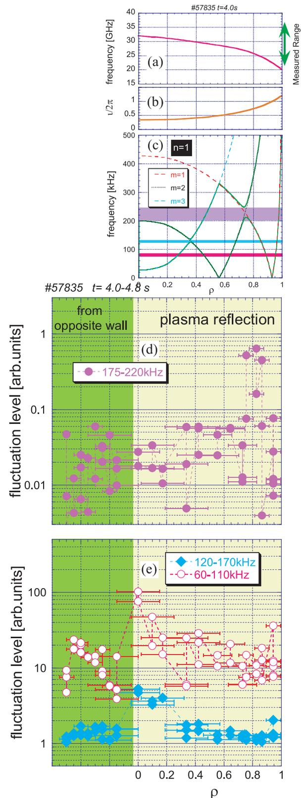
Fig. 6 Radial profiles of (a) right-hand cutoff frequency, (b) iota, and (c) Shear Alfvén spectra for  $n = 1$ . Radial profiles of fluctuation component, obtained by *Ka*-band Hopping reflectometer, which is integrated in the frequency ranges of (d) 175-220 kHz, and (e) both 120-170 kHz and 60-110 kHz, respectively.
