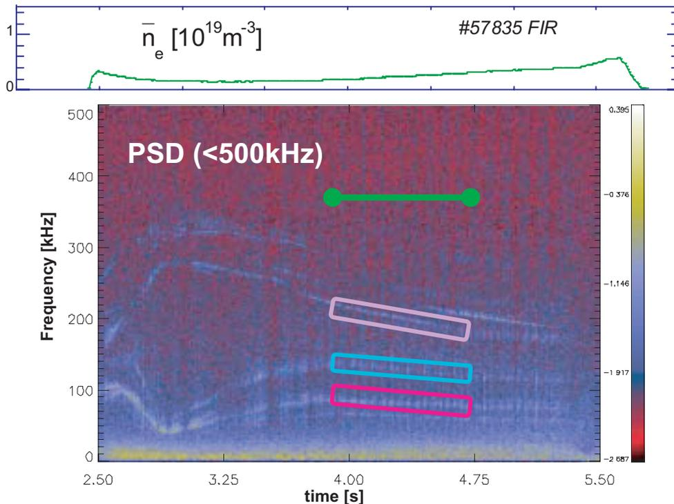
Fig. 5 Time evolution of electron density and frequency spectrum of interferometer mode CW Reflectometer.
