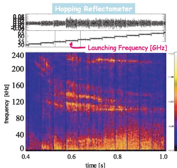
Fig. 8 Temporal behavior of the Frequency Hopping V-band Reflectometer signal and its frequency spectra.
