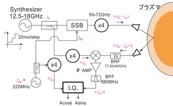
Fig. 7 Schematic view of Frequency Hopping V-band Reflectometer system.
