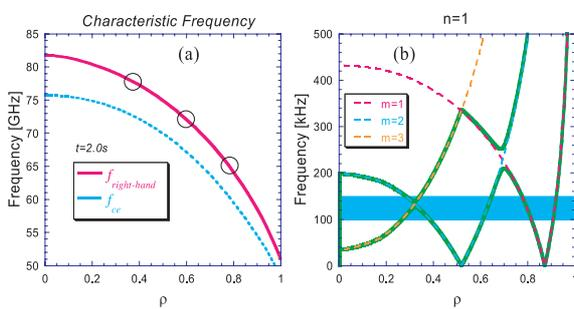
Fig. 1 (a) Radial profiles of right-hand cut-off frequency (red solid line) and electron cyclotron frequency (blue dotted line) (b) Radial profile of shear Alfvén spectra for  $n = 1$ .
