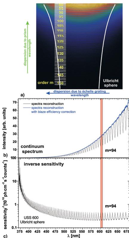
Fig. 3 Radiometric calibration of the cross-dispersion spectrometer. (a) 2D image of the system during exposure by a continuum light source. (b) Complete reconstructed spectrum of the continuum spectrum. Intensity drops caused by the blaze angle dependence of the grating are considered in the calibration by a correction function. (c) Spectral response of the system for the full wavelength span.
