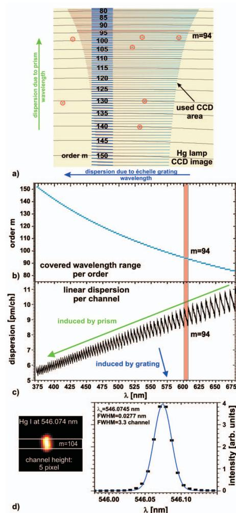
Fig. 2 Spectrum reconstruction: (a) 2D image of a Hg line spectrum. The spectral range per order applied for the complete spectrum reconstruction is represented by the envelope. (b) Distribution of the wavelength coverage per order. (c) Linear dispersion over the full spectral range. (d) A HgI line is used to approximate the apparatus function.
