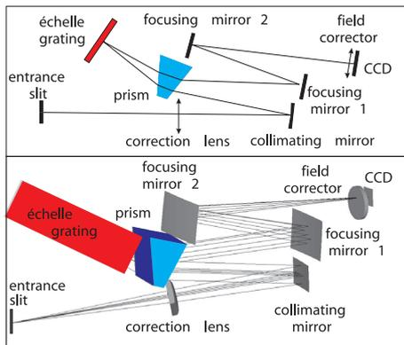
Fig. 1 (a) Schematic view of the spectrometer set-up. (b) Ray tracing calculation showing the optical path in the spectrometer. The optical elements are to scale.
