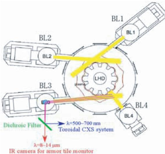
Fig. 1 Arrangement of three high-energy tangential NB injectors (BL1, BL2, and BL3) and a low-energy perpendicular NB injector (BL4). A toroidal line of sight from the BL3-injection port for the CXS system, which utilizes the BL4 beam, is also indicated.
