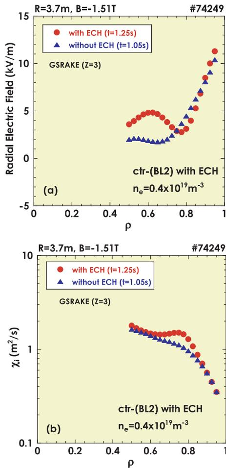
Fig. 4 Results of the neoclassical calculation using the GSRake code for the plasmas with and without the ECRH superposition shown in Fig. 2 (a). Radial electric-field profiles and (b) ion thermal-diffusivity profiles.
