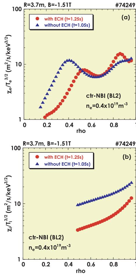
Fig. 3 Profiles of (a) electron thermal diffusivities normalized by  $T_e^{3/2}$ ,  $\chi_e/T_e^{3/2}$ , and (b) ion thermal diffusivities normalized by  $T_i^{3/2}$ ,  $\chi_i/T_i^{3/2}$ , for the NBI plasmas with and without the ECRH superposition shown in Fig. 2.
