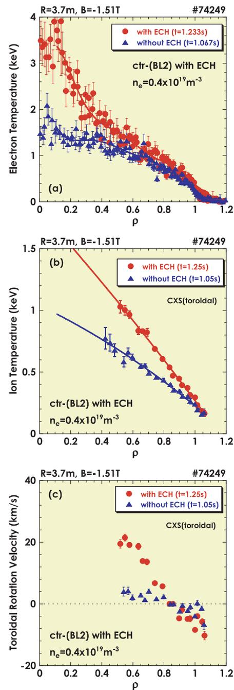
Fig. 2 (a) Electron temperature profiles, (b) ion temperature profiles, and (c) toroidal rotation velocity profiles, with and without ECRH superposition to the plasmas heated with both the counter-NBI (BL2) and the perpendicular-NBI (BL4). While the electron temperature profiles are polynomially fitted, the ion temperature profiles are parabolically extrapolated to the center.
