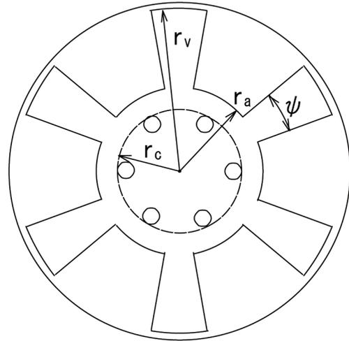
Fig. 2 Schematic of a magnetron.
