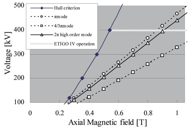
Fig. 3 Magnetron operating region.
