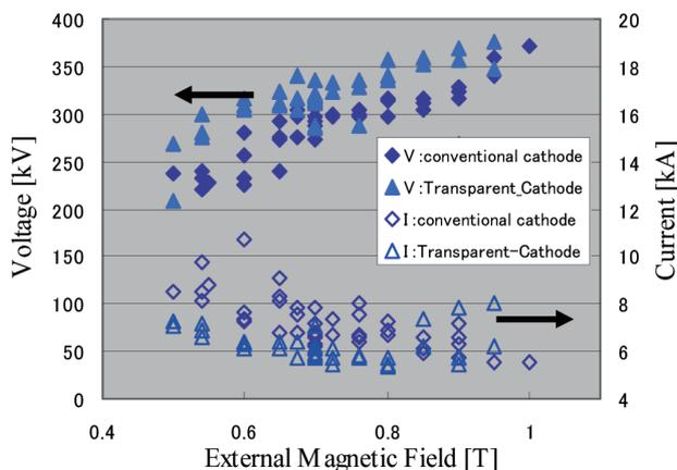
Fig. 4 Voltage-current characteristics of the magnetron as a function of magnetic field. The diamond dots denote measured values with the traditional cathode. The triangle dots denote measured values with the transparent cathode.
