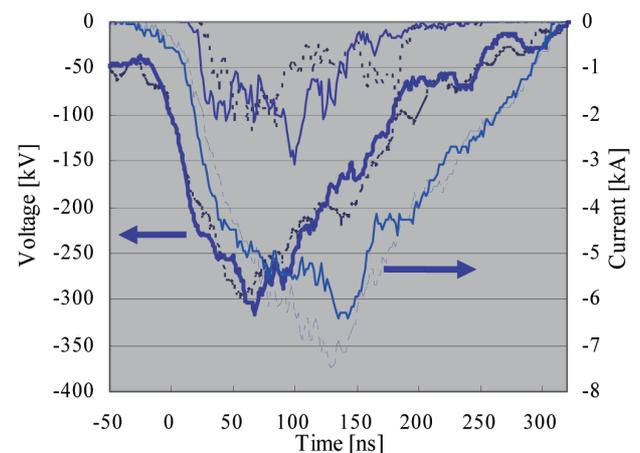
Fig. 5 Voltage, current, and microwave pulses at 0.76 T. Full lines show operation with the transparent cathode. Dashed lines show operation with the traditional cathode. Heavy lines represent the diode voltage. Normal lines represent the diode current. Top lines represent the microwave pulses.
