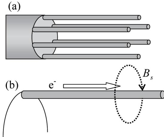
Fig. 1 Transparent cathode model showing the independent cathode strips (a), and the magnetic effect near a strip (b).
