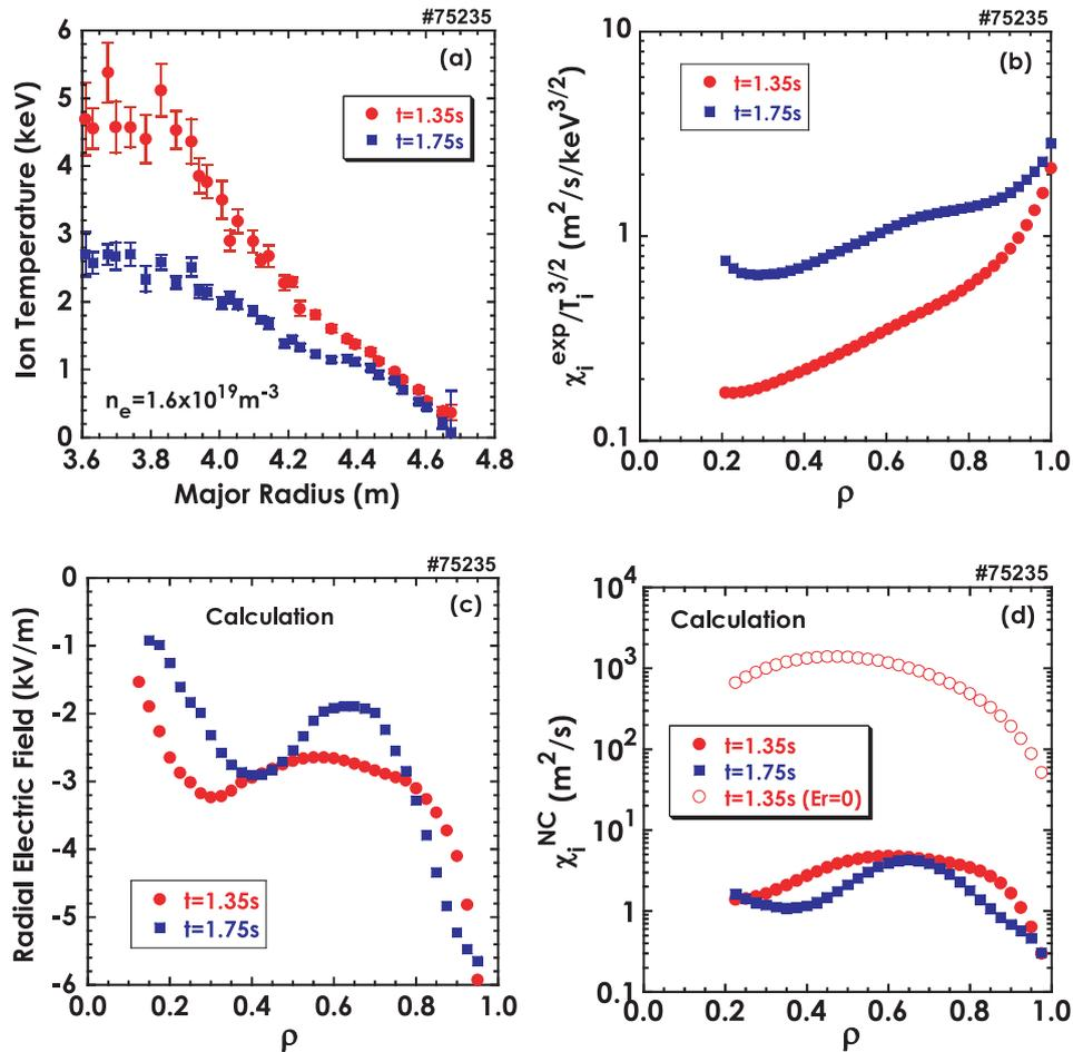
Fig. 8 (a)  $T_i$  profiles in the plasmas used for the transport analysis, and (b) the obtained experimental ion thermal diffusivities divided by the gyro-Bohm factor,  $\chi_i/\Gamma_i^{3/2}$ . (c) Radial electric field,  $E_r$ , and (d) the neoclassical ion thermal diffusivities,  $\chi_i$ , estimated with the neoclassical ambipolar calculation for the plasmas in (a). In (d),  $\chi_i$  without consideration of the  $E_r$  effect is also indicated.
