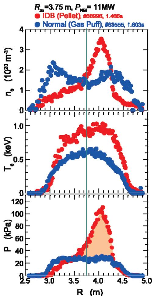
Fig. 6 Comparison of electron density, electron temperature, and plasma pressure profiles of the SDC/IDB plasma with those of the gas-puffing plasma with no IDB [22]. The preset vacuum-magnetic axis position of  $R_{ax}^{vac} = 3.75$  m is indicated by a vertical line. The magnetic field strength and NBI power for both plasmas are the same, 2.539 T and 11 MW, respectively.
