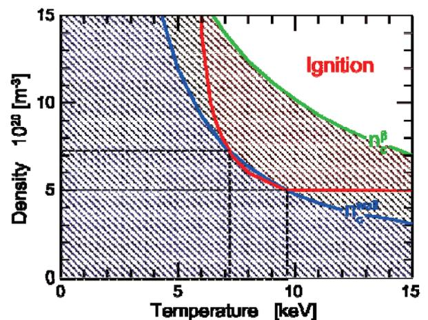
Fig. 9 Operational regime of central density and temperature for high-density ignition in the helical reactor based on the IDB profile. The lines of  $n_c^{wall}$  and  $n_c^\beta$  indicate critical boundaries for a neutron wall loading less than  $2 \text{ MW/m}^2$  and a central beta less than 7%, respectively.
