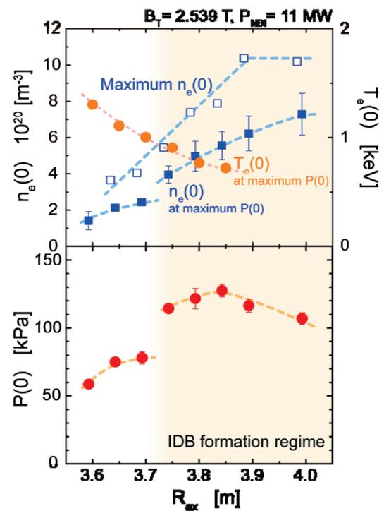
Fig. 5 Maximum central electron density,  $n_e(0)$ , and maximum plasma pressure,  $P(0)$ , obtained at various preset vacuum-magnetic axis positions,  $R_{ax}^{vac}$  [23]. Top: maximum  $n_e(0)$  together with  $n_e(0)$  and  $T_e(0)$  at maximum  $P(0)$  as a function of  $R_{ax}^{vac}$ . Bottom: maximum  $P(0)$  as a function of  $R_{ax}^{vac}$ .
