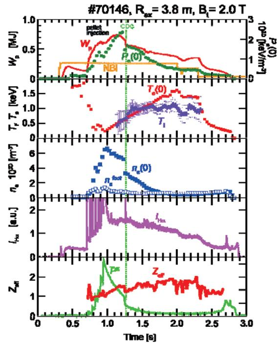
Fig. 4 Typical waveforms of the SDC/IDB plasma formed in the HD configuration. From top: stored energy,  $W_p$ , and central electron pressure,  $P_e(0)$ , electron and ion temperatures, central and peripheral (foot) electron densities,  $H_\alpha$  intensity, and effective  $Z$ , and Bremsstrahlung radiation power.
