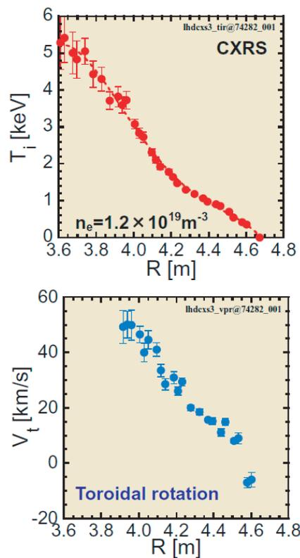
Fig. 7 Profiles of the ion temperature and toroidal rotation velocity in the high- $T_i$  plasma heated with a combination of low-energy and high-energy NBIs. The magnetic axis position is 3.575 m, magnetic field strength is 2.77 T, and electron density is  $1.2 \times 10^{19} \text{ m}^{-3}$ .
