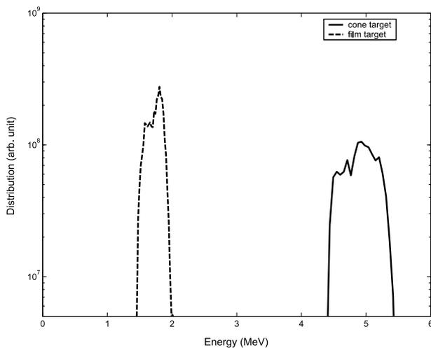
Fig. 4 Energy spectra of protons at  $t = 70\tau_0$  for the cone target (solid line) and film target (dashed line).
