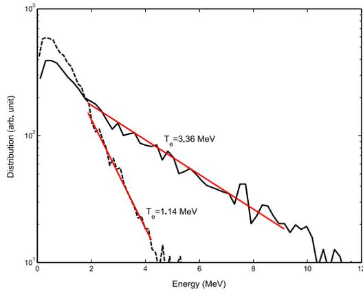
Fig. 3 Energy spectra of electrons escaping from the rear surface of the cone target (solid line) and film target (dashed line).
