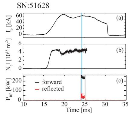
Fig. 2 Typical RF heated discharge. (a) plasma current, (b) line-integrated density, (c) RF power. The blue vertical line shows the laser injection timing ( $t = 24.37$  ms).
