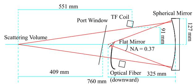
Fig. 1 Configuration of the collection optics.
