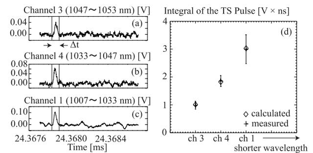
Fig. 3 (a)~(c) Output signals of three channels of the polychromator measured at  $R = 380$  mm (SN51628). Black vertical lines show the integration interval  $\Delta t = 60$  ns. (d) Measured and calculated signals of each polychromator channel.  $T_e = 210$  eV and  $n_e = 2.14 \times 10^{19} \text{ m}^{-3}$  were used for the calculation (diamonds in Fig. (d)).
