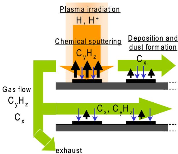
Fig. 4 Schematic illustration of erosion and dust formation.
