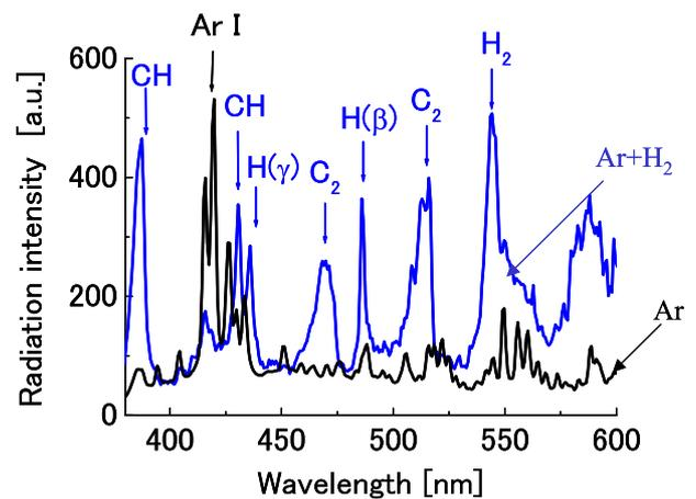
Fig. 2 Radiation spectra at 5 mm above graphite target 1 during Ar (black line) and Ar/H<sub>2</sub> (blue line) plasma irradiation.
