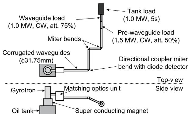
Fig. 2 Schematic view of the experimental set up.
