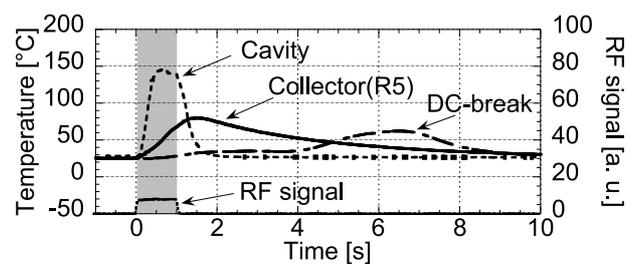
Fig. 4 Time evolution of DC-break cooling water temperature and temperatures measured by thermocouples at the cavity and the middle-part of the collector.
