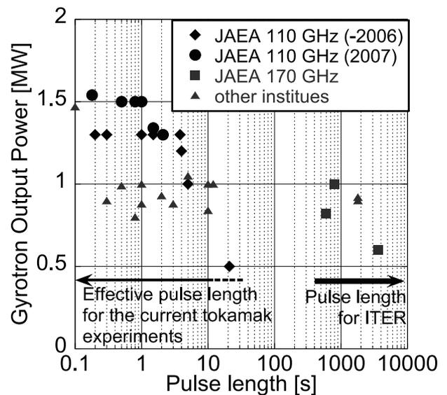
Fig. 1 Gyrotron output power vs. pulse length (> 0.1 s) achieved in the world.
