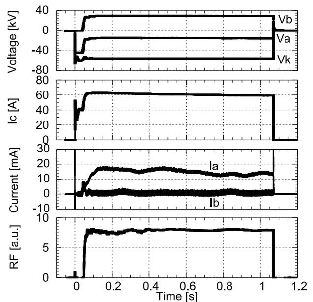
Fig. 3 Time evolution of the voltages on cathode ( $V_k$ ), anode ( $V_a$ ) and body ( $V_b$ ), the currents on collector ( $I_c$ ), anode ( $I_a$ ) and body ( $I_b$ ), and the RF signal detected at the directional coupler.
