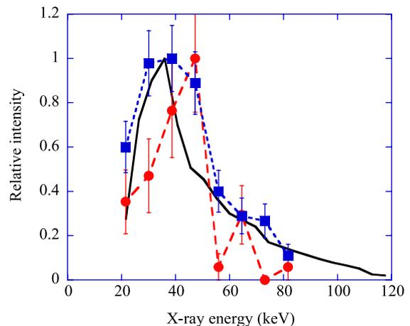
Fig. 4 Backscattered spectrum shifts from the primary X-ray. Solid line: Primary X-ray. Circle: Lead of 20 mm thickness. Square: Acrylic of 30 mm thickness.
