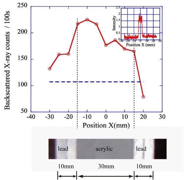
Fig. 3 Upper: Backscatter X-ray imaging. The top right window is the primary X-ray shape. Lower: Structure of the scattering material. Circles indicate the experimental results. Horizontal dashed line indicates the background level. Vertical lines correspond to the boundary between the lead and the acrylic, as shown in the bottom.
