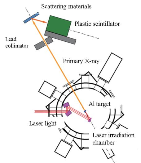
Fig. 1 Schematic setup for measurement of backscattered X-ray intensity.
