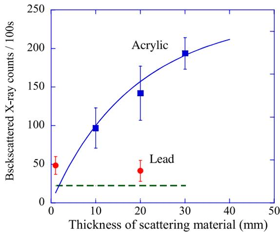
Fig. 2 Dependence of backscattered X-ray counts on scattering materials and their thickness. Dashed line indicates the background level. Solid line indicates the theoretical model for acrylic.
