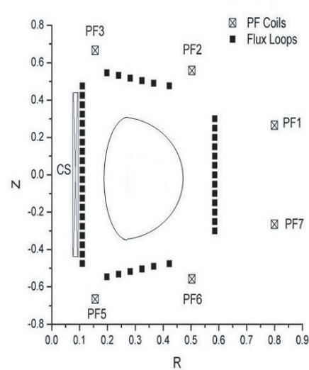
Fig. 2 Magnetic sensor positions of CPD.
