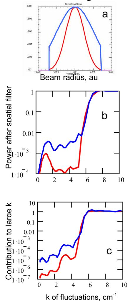
Fig. 3 Attenuation of PCI signal vs wavelength of the plasma wave. (a) Beams profiles at the input port; (b) total power of the PCI signal after spatial filter and phase plate; (c) high k contribution.
