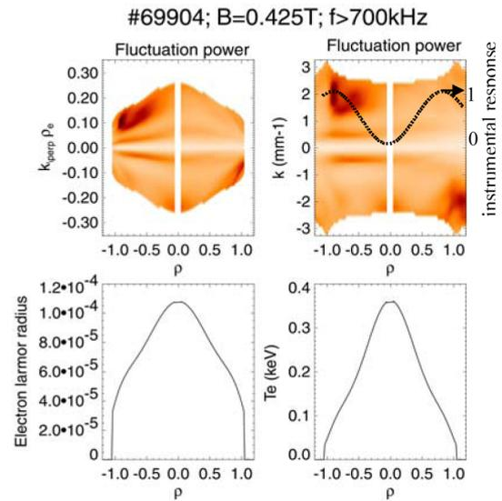
Fig. 2 Profile of density fluctuations with large  $k$  observed in discharge with low magnetic field. The dashed black curve shows instrumental response for  $k = 2 \text{ mm}^{-1}$ , which has a minimum in the plasma center.
