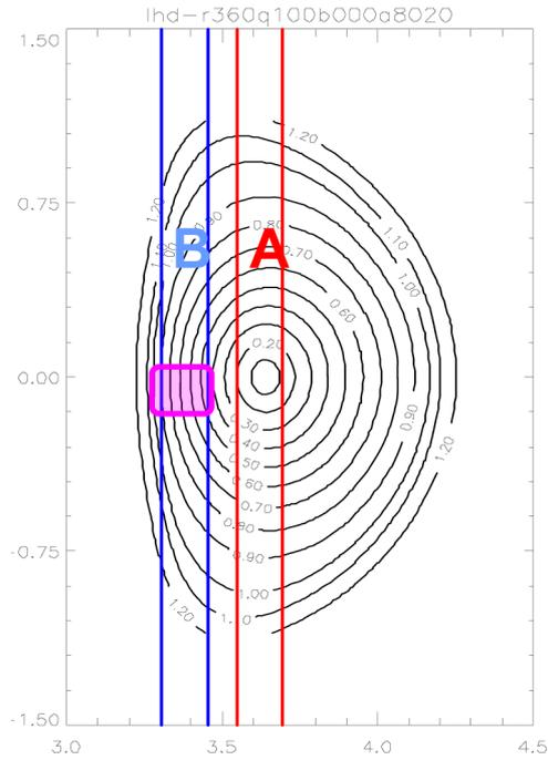
Fig. 1 Geometry of present PCI probe beam (A, red) shown for magnetic configuration with axis position  $R_{ax}=3.6$  m and  $\beta = 0$ .
