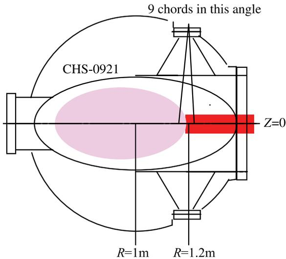
Fig. 1 Geometrical location of the outermost flux surface and the vertically viewing chords in the vacuum vessel at the horizontally elongated sections.
