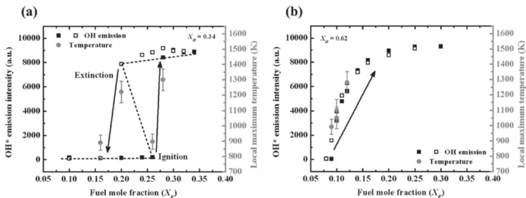
Fig. 9 Relationship between OH\* emission intensity, local maximum temperature and fuel mole fraction,  $f = 24$  kHz,  $a = 400$  1/s, (a)  $X_O = 0.34$ , (b)  $X_O = 0.62$ , (solid square symbols: increasing  $X_F$ , open square symbols: decreasing  $X_F$ ).
