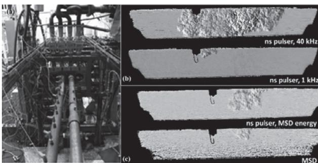
Fig. 2 (a) PDE engine facility at the Air Force Research Lab at Wright-Patterson Air Force Base, (b) Schlieren imaging of nanosecond pulsed discharge igniter in CH<sub>4</sub>/air mixture,  $\Phi=1$ , (c) Schlieren imaging of nanosecond pulsed discharge igniter in CH<sub>4</sub>/air mixture,  $\Phi=0.8$  [22].
