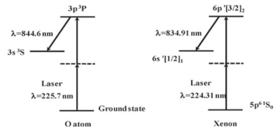
Fig. 10 Schematic of atomic O and Xenon atom energy levels with two photon absorption excitation and fluorescence schematic [64].
