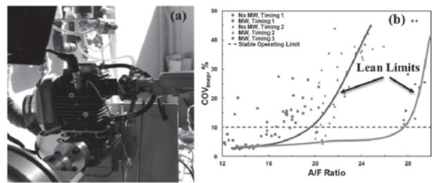
**Fig. 1** (a) Direct photograph of plasma assisted 34 cc Fuji engine test setup and (b) the comparison of limits of stable engine operating conditions with and without microwave (MW) discharge [17].
