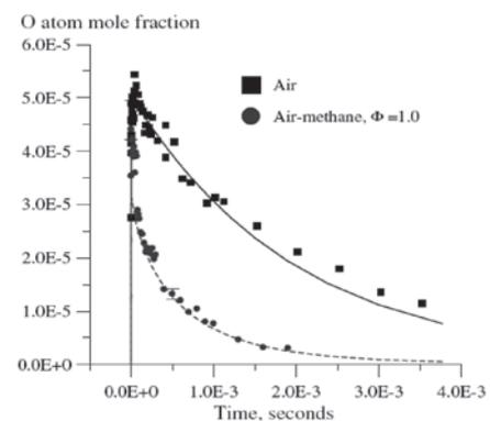
Fig. 11 Atomic O mole fraction vs. time after a single high-voltage pulse in air and in a methane-air mixture at  $P = 60$  torr and  $\phi = 1.0$  [51].
