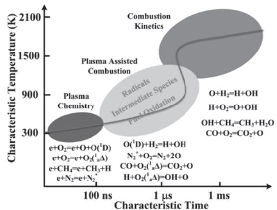
Fig. 6 Kinetic regimes and timescales of a typical plasma assisted combustion process.
