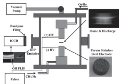
Fig. 8 Schematic of experimental setup integrating counterflow system with *in situ* discharge.
