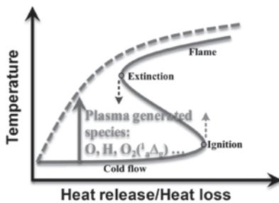
Fig. 4 Schematic of the classical ignition and extinction S-curve (solid line) and the stretched S-curve (dashed line).
