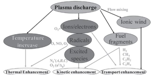
Fig. 5 Possible enhancement pathways of plasma on combustion systems.
