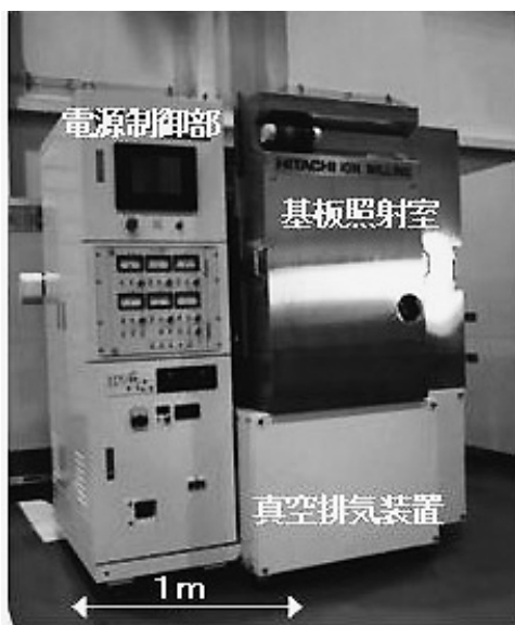
Fig. 2 Photo of ion beam milling system (The photo offered by AE KiKi Engineering Co Ltd.).
