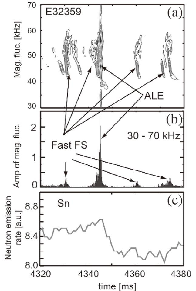
Fig. 1 Temporal evolutions of (a) frequency spectrum of magnetic fluctuations measured by Mirnov coil, (b) amplitude of magnetic fluctuations with frequency of 30 – 70 kHz, (c) neutron emission rate.
