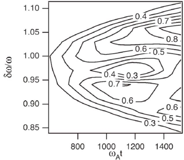
Fig. 3 Temporal evolution of frequency spectrum of radial magnetic field fluctuations in simulation by MEGA code.
