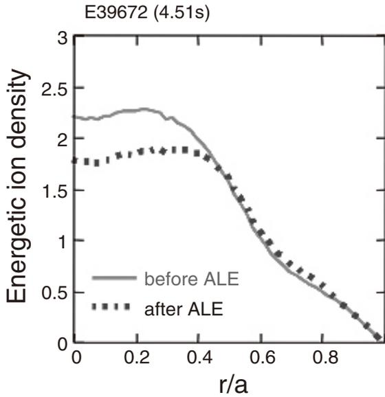
Fig. 2 Fast ion density profiles before and after ALE. These profiles are derived from the data obtained by a neutron profile monitor.
