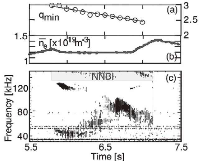
Fig. 6 (a) Temporal evolution of  $q_{\min}$ , (b) line averaged electron density, (c) a time trace of frequency spectrum of the  $n = 1$  instability. Note: three horizontal vague lines around 48 kHz and 36 kHz in the figure come from noise in Mirnov coil system.
