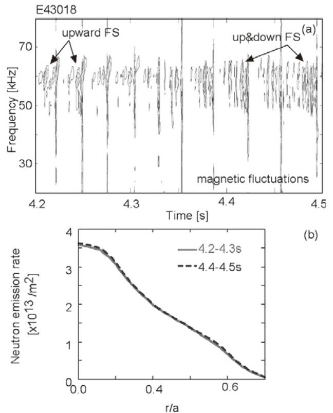
Fig. 4 (a) Temporal evolution of frequency spectrum of magnetic fluctuations. (b) Time averaged neutron emission profiles measured by neutron profile monitor for two time intervals of  $t = 4.2\text{s}$  to  $4.3\text{s}$  and  $t = 4.4\text{s}$  to  $4.5\text{s}$ .
