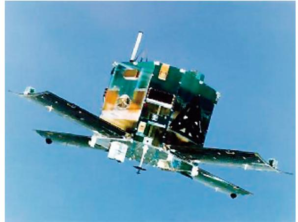
Fig. 2.6.6 Scientific satellite “AKEBONO” and two circular electrodes which are attached at the end of solar cell paddles.
