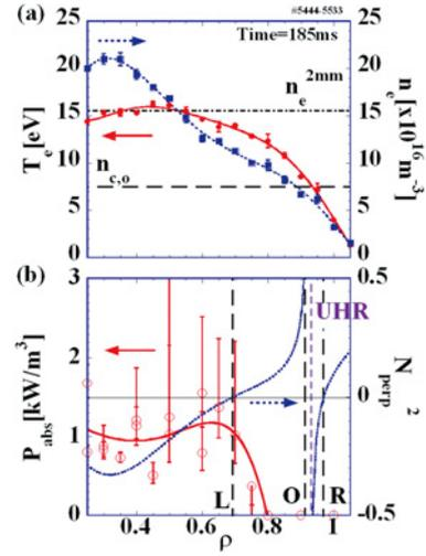
Fig. 3 (a) Radial profiles of  $T_e$  and  $n_e$  at  $t = 185$  ms. (b)  $P_{abs}$  and squared refractive index ( $N_{perp}^2$ ). Signs, such as O, R, L and UHR, respectively stand for the layers of O-mode cutoff, right-hand cutoff, the left-hand cutoff, and upper hybrid resonance.
