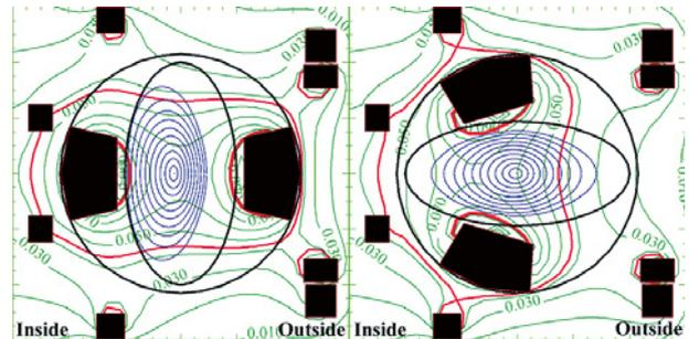
Fig. 1 Contours of the magnetic field strength and magnetic surfaces of CHS plasma at  $B_t = 0.0613$  T and  $R_{ax} = 97.4$  cm. The thick and thin red curves indicate the fundamental ECR and 2nd harmonic layers respectively.
