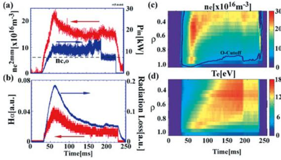
Fig. 2 (a) and (b): Time evolutions of  $n_e^{2mm}$ ,  $P_{in}$ ,  $H\alpha$  and total radiation loss. (c) and (d): Contour plots of  $n_e$  and  $T_e$  in time and normalized radius ( $\rho$ ) plane. The solid curve in (c) indicates O-mode cutoff density ( $n_{c,o}$ ).
