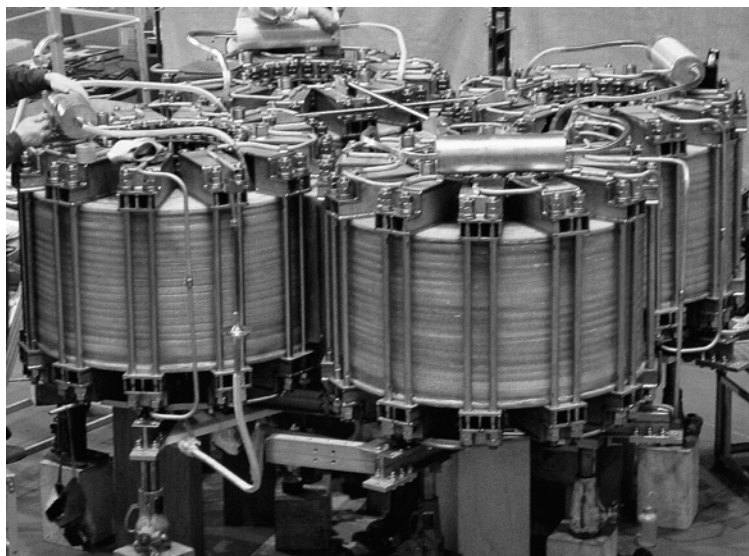
Fig. 5 Photograph of SMES model coil in National SMES project II.
