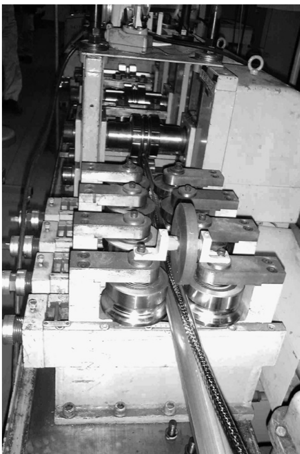
Fig. 6 Conduit forming process of cable-in-conduit conductor.
