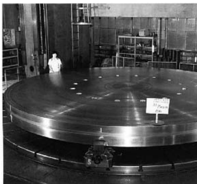
Flywheel on Machining D = 6\text{ m} , t = 0.4\text{ m} , Weight = 107 t, one disk of the six disks bolted flywheel
