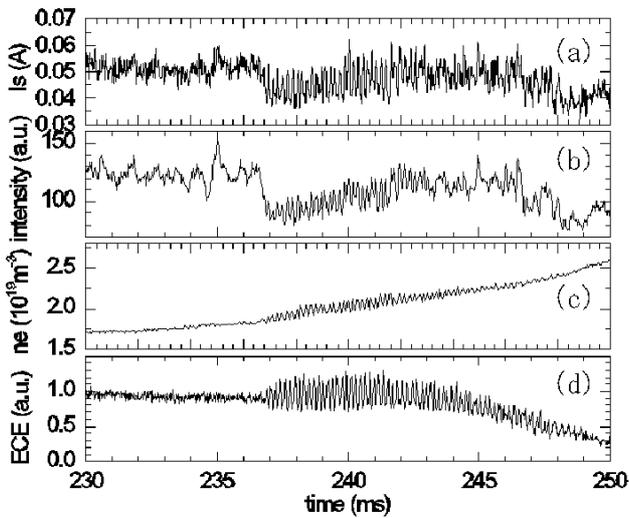
Fig. 3 (a) Ion saturation current of the Langmuir probe on the limiter head, (b)  $H_{\alpha}$  signal of pixel data at the probe position in the fast camera images, (c) Line-average electron density, (d) ECE signal from the plasma central region.
