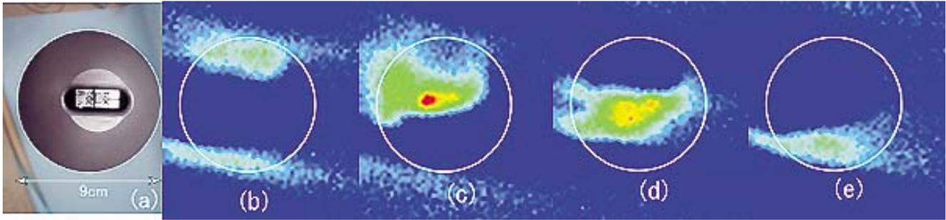
Fig. 2 (a) Top view of carbon limiter, in central region there are 4 Langmuir probes; each two is separated by a block of SiC. (b-e) Two-dimensional contour images at a 5.7 kHz frequency spectral power obtained by FFT during fluctuation period. Each frame continues in this order at every 49.4  $\mu$ sec. In (b-e) the white circle shows the outline of the carbon limiter.
