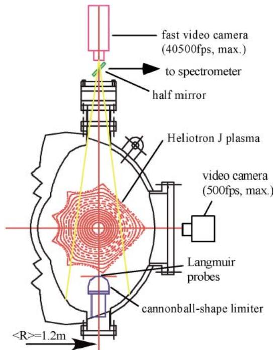
Fig. 1 Experimental setup in Heliotron J for new limiter experiments.
