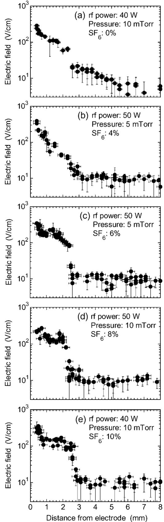
Fig. 1 Distributions of electric field measured at various percentages of SF<sub>6</sub> in Ar/SF<sub>6</sub> inductively-coupled plasmas.
