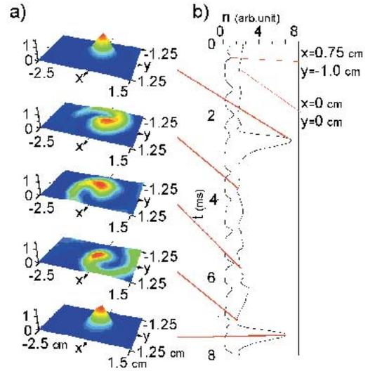
Fig. 3 Ion transport pulsation. a) Two-dimensional density profiles. b) Temporal behavior of pulsation.
