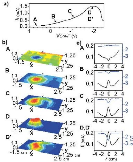
Fig. 2 Plasma behaviors as a parameter of the well potential ( $V_{\text{Col-E}} < 0$ ). a) Ion current of the probe at  $r = 0$ . b) Density profiles on a plane perpendicular to the magnetic field. c) Time averaged density and potential versus radial position. Each figure of b) and c) corresponds to the positions A, B, C and D (D') of a).
