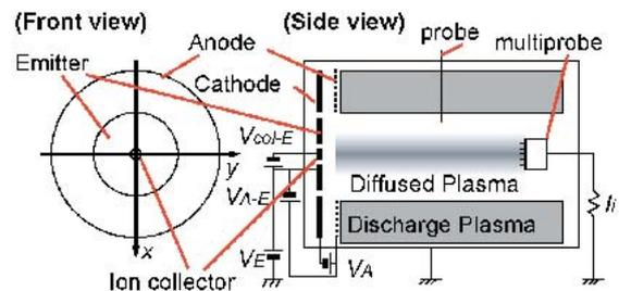
Fig. 1 Experimental apparatus. A diffused plasma is formed inside a discharged hollow plasma. Ions are accumulated around the central axis by a negative voltage of the ion collector.
