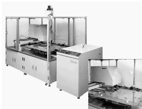
Fig. 2 Aiplasma for large-size LCD panels and PC boards.
