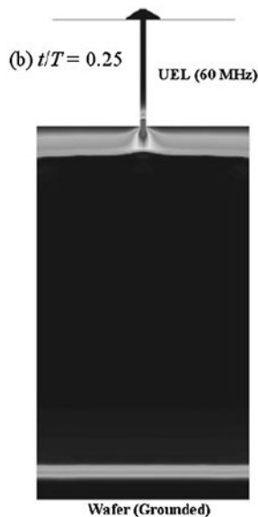
図 1 イオン化レート (1/4 周期, ガス流量 0.9 sccm). (Reprinted from "Locally enhanced discharges at gas hole outlets of a showerhead in a plasma etching reactor", K. Denpoh 2009 J. Phys. D: Appl. Phys 42, 032003 (2009), © IOP Publishing. Reproduced with permission. All rights reserved)
