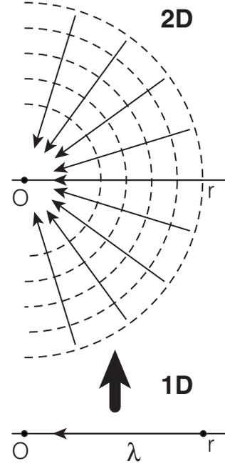
Fig. 1 Illustration of a wrong modeling of first-generation neutral trajectories, denoted by slim arrows, born at the magnetic surface  $r$ . The magnetic surface is denoted by the broken line and the magnetic axis by  $O$ .
