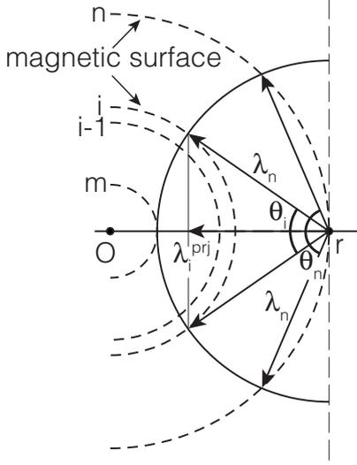
Fig. 2 Illustration of the computation of an effective mean free path of a first-generation neutral at a position  $r$ , corresponding to the magnetic surface denoted by  $n$ . A mean free path is denoted by  $\lambda$  and an angle between the intersection points of a magnetic surface and a neutral trajectory by  $\theta$ . The subscripts correspond to the labels of the magnetic surface.
