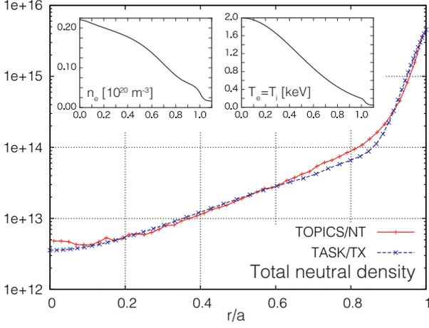
Fig. 3 Comparison of the neutral density profile calculated by a Monte Carlo code TOPICS/NT with that by TASK/TX in a transient phase at  $t = 0.1$  s, in the lower plasma density case.
